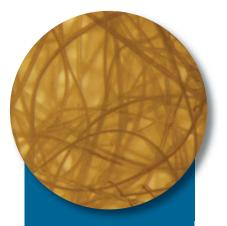
Thinsulate<sup>™</sup> Insulation FR has lofty fibrous webs that trap more air and contain more of the body's radiant heat than higher-density traditional needle-punched webs.
